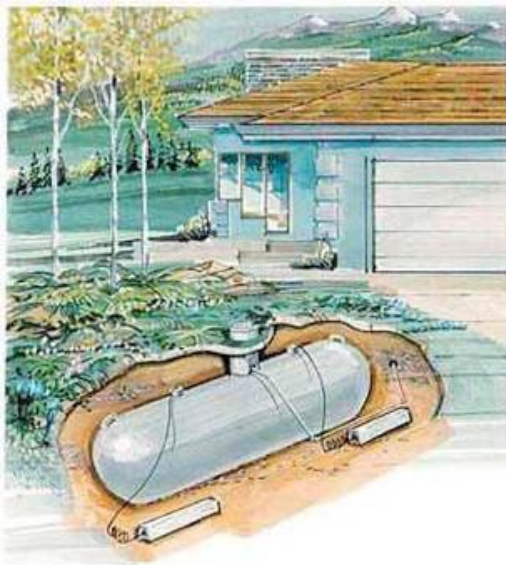
Propane tank with cathodic protection
